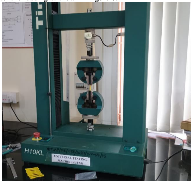
Figure 6: Tensile Specimen Placed in UTM
